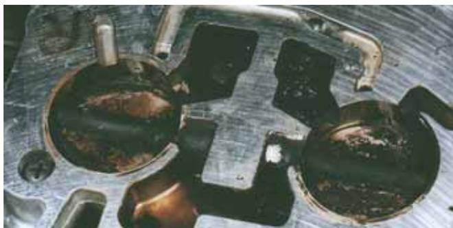
**Picture J** - Carburetor plates before P.i. treatment
