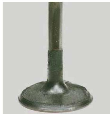
**Picture E** - Intake valve after P.i. treatment
